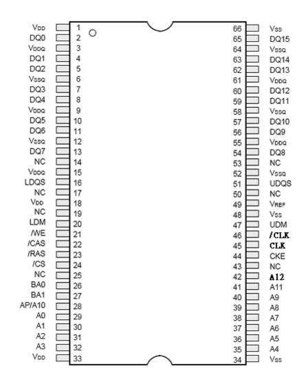
66pin TSOP-II / (400mil × 875mil) / (0.65mm Pin pitch)
